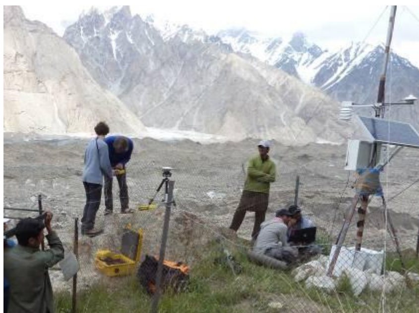
Exhibit 16 The GPS Master station located at Urdukas (Baltoro Glacier). In 2011 it was used as reference station to evaluate stake positions and then glacier surface velocity (the measurements were acquired twice, at the beginning and the end of the field work thus permitting a comparison of the surveyed data). The GPS Master station was located close to the Share AWS (on the right in the photo provided by C Mayer).
