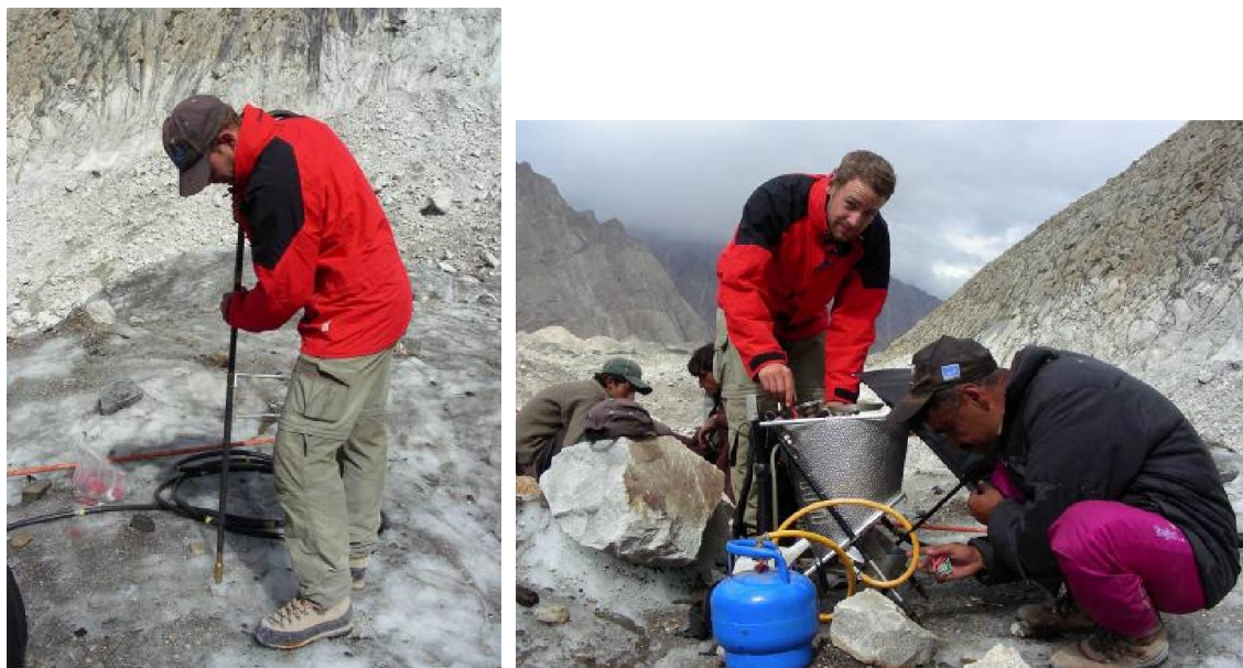
Exhibit 7 Drilling an ablation stake with the Heucke steam drill at Khoburtse Glacier (Photos by C Mayer)
