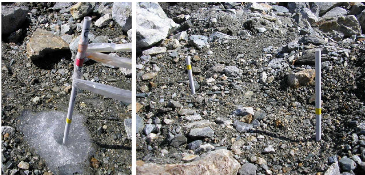
Exhibit 18 Stake farm to measure ice ablation with varying debris thickness (Photos by C Mihalcea).
