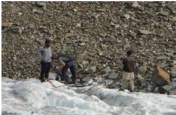
Exhibit 6 Drilling an ablation stake with the Heucke steam drill at Concordia – Baltoro Glacier (Photos by C Mayer)
