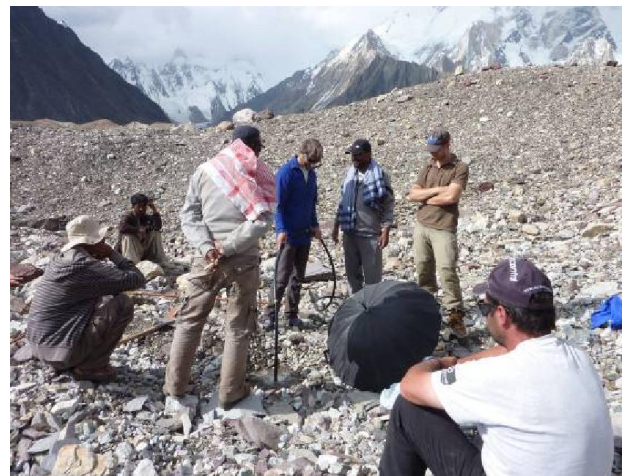
Exhibit 6 Drilling an ablation stake with the Heucke steam drill at Concordia – Baltoro Glacier (Photos by C Mayer)
