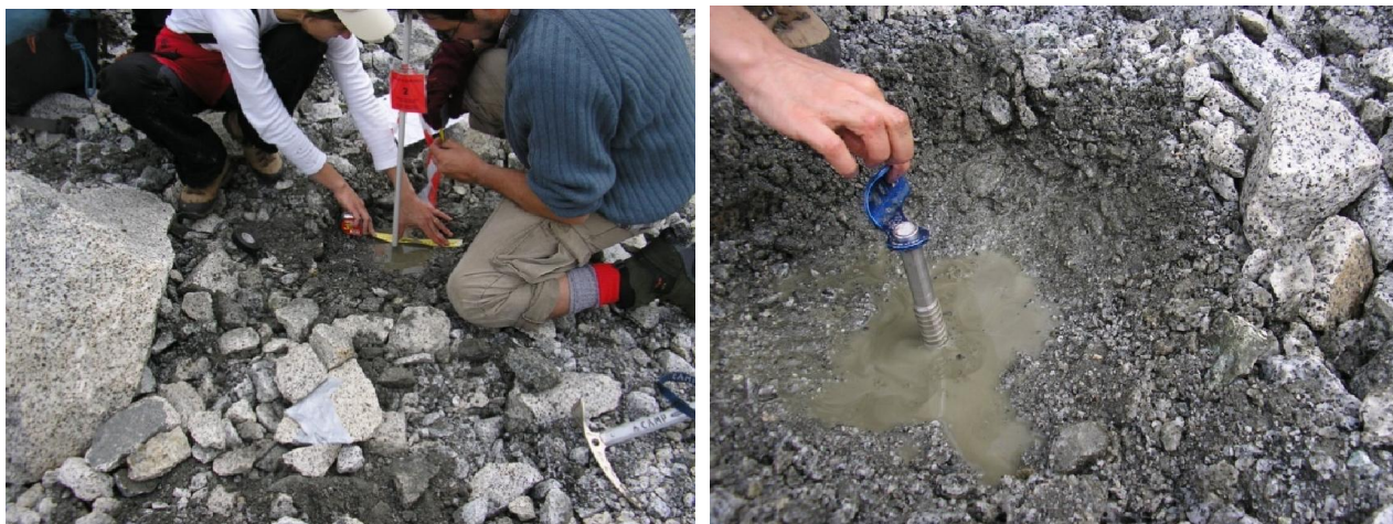
Exhibit 17 Installing ice ablation stakes on debris-covered ice (Photos by C Mihalcea)
