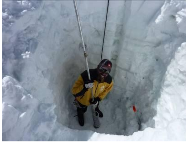
Exhibit 11 Digging a snowpit (see the vertical profile for snow layer analysis and sampling) at the Godwin Austen basin (Photo by C Mayer).
