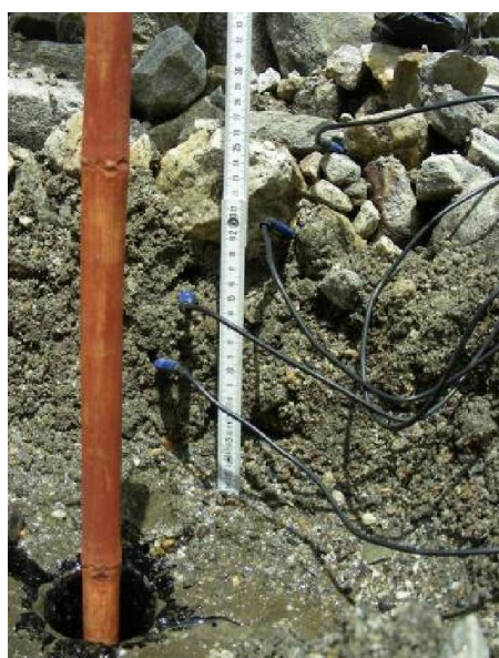
Exhibit 9 An ablation stake installed at at Khoburtse Glacier. This stake is also equipped with thermistors and data loggers to record debris temperature data along the debris vertical profile (Photo by C Mayer)
