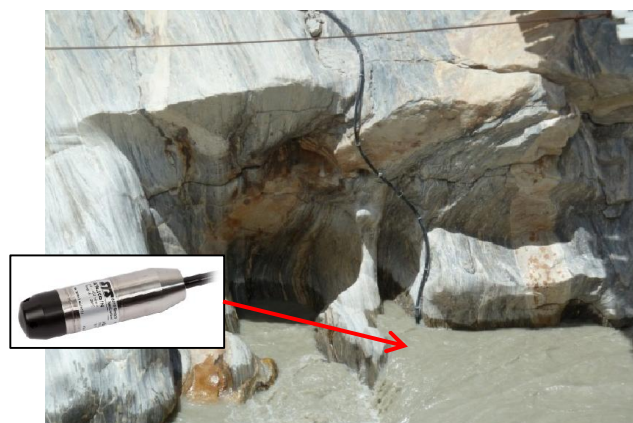
Exhibit 28: Pressure transducer mounted at the bridge near Paiju.
