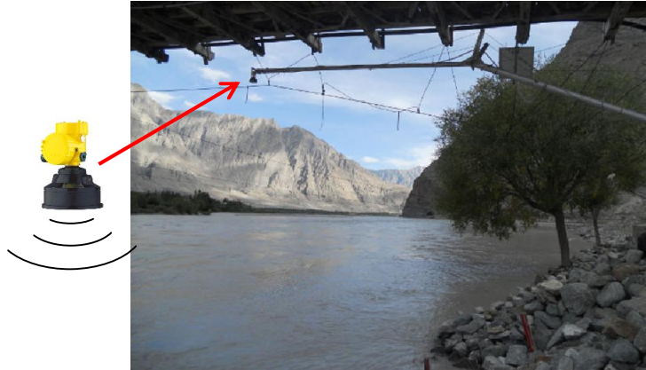
Exhibit 29: Sonic sensor mounted at Shigar's bridge.
