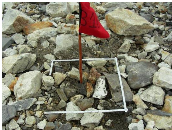
Exhibit 8 A bamboo ablation stake installed at Khoburtse Glacier (Photo by C Mayer)
